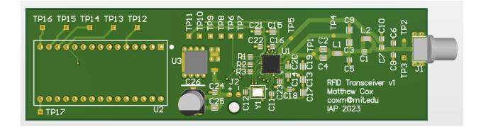
It's a four-layer PCB. where the top layer is components and signal, the 2nd layer is ground, the 3rd layer is +5V power, and the bottom layer is another signal layer.
