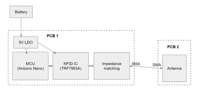
Here's a schematic of the main board:
