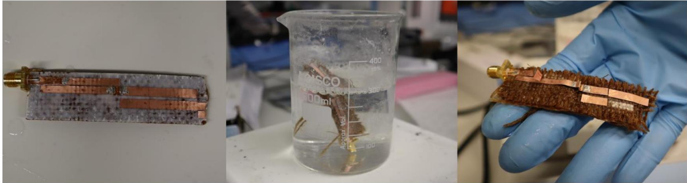
Figure 8. Dissolving the microstrip filter in water and the remaining natural fibres and delaminated copper tracks.
