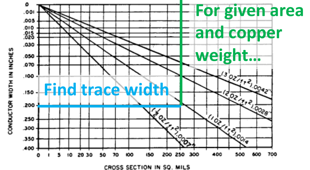
Figure B Conductor width to cross-section relationship
