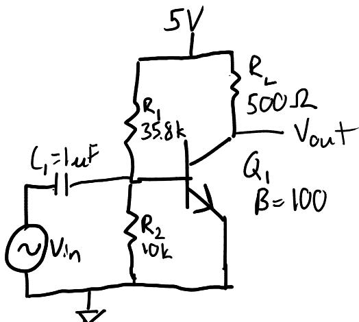
Our goal is to calculate the gain of this common-emitter amp. We will assume  $V_{BE} = 0.7V$ , which is often a safe assumption that is guaranteed by the device properties of the BJT.
