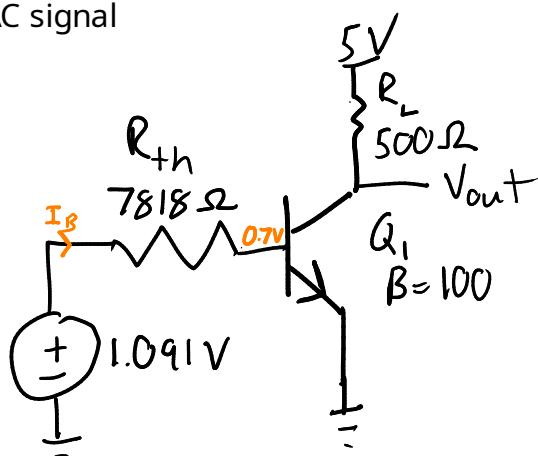
Now, using the assumption that  $V_{BE}=0.7V$
